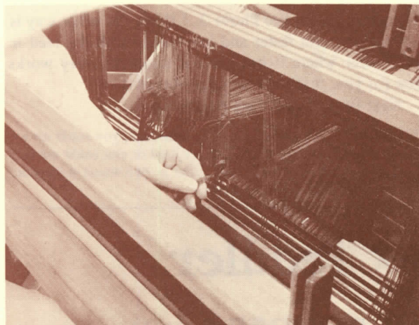
Photo 1—Threaded heddles are pushed to the left. The group you are working with is pulled to the right so there is plenty of space for handling.
